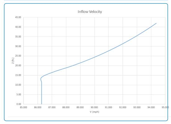
**Figure 2:** Inflow velocity according to ASCE/SEI 7-16 (exposure category D, basic wind speed 100 mph)
