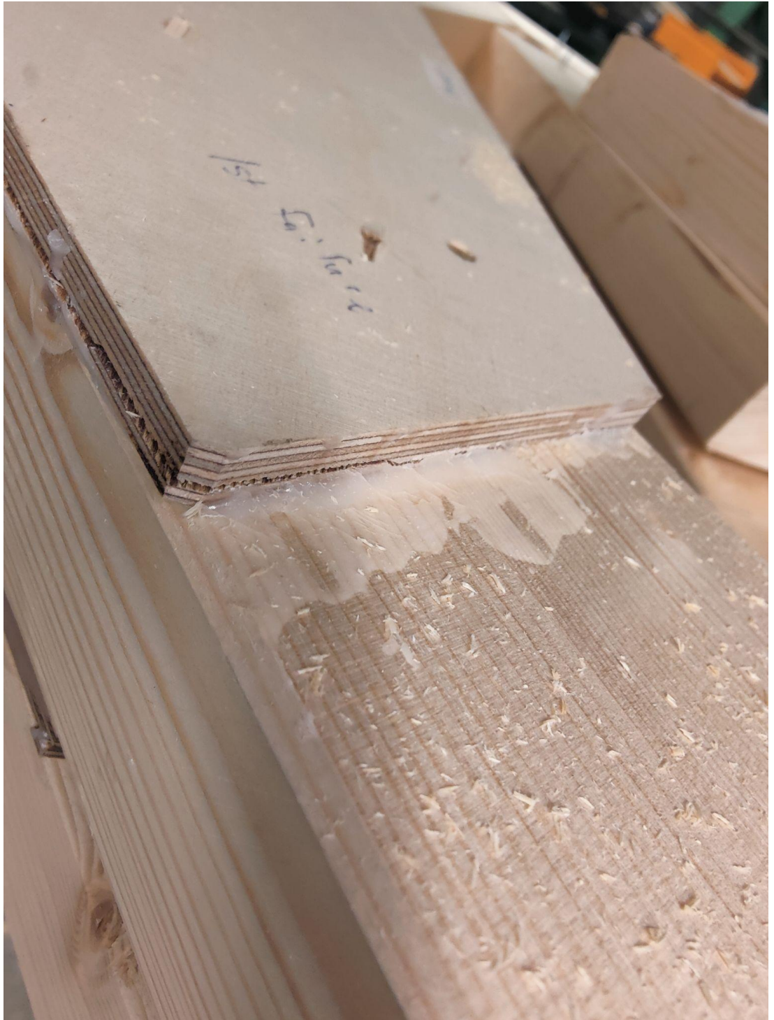
Figure A1.17.5 Delamination at gusset plates, 1st failure
