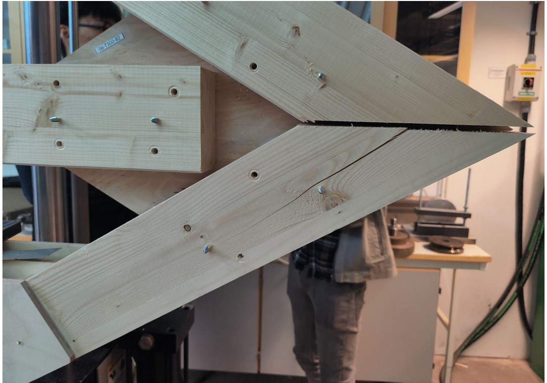
Figure A1.6.3. Timber failure in diagonal of specimen 6
