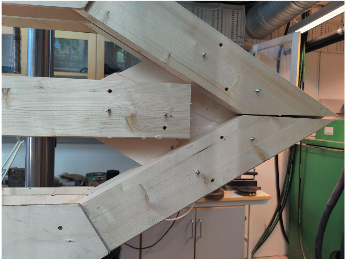
Figure A1.17.3 Tension/shear failure in plywood
