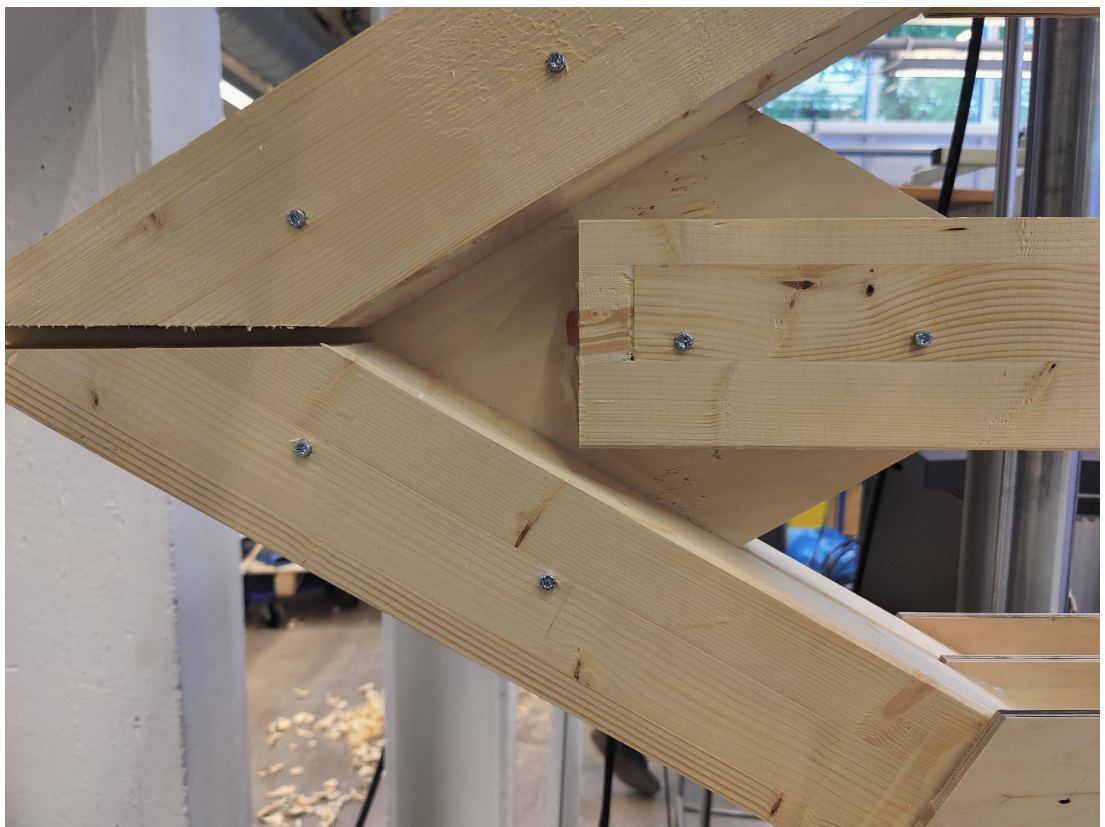
Figure A1.14.4 Tensile failure in plywood
