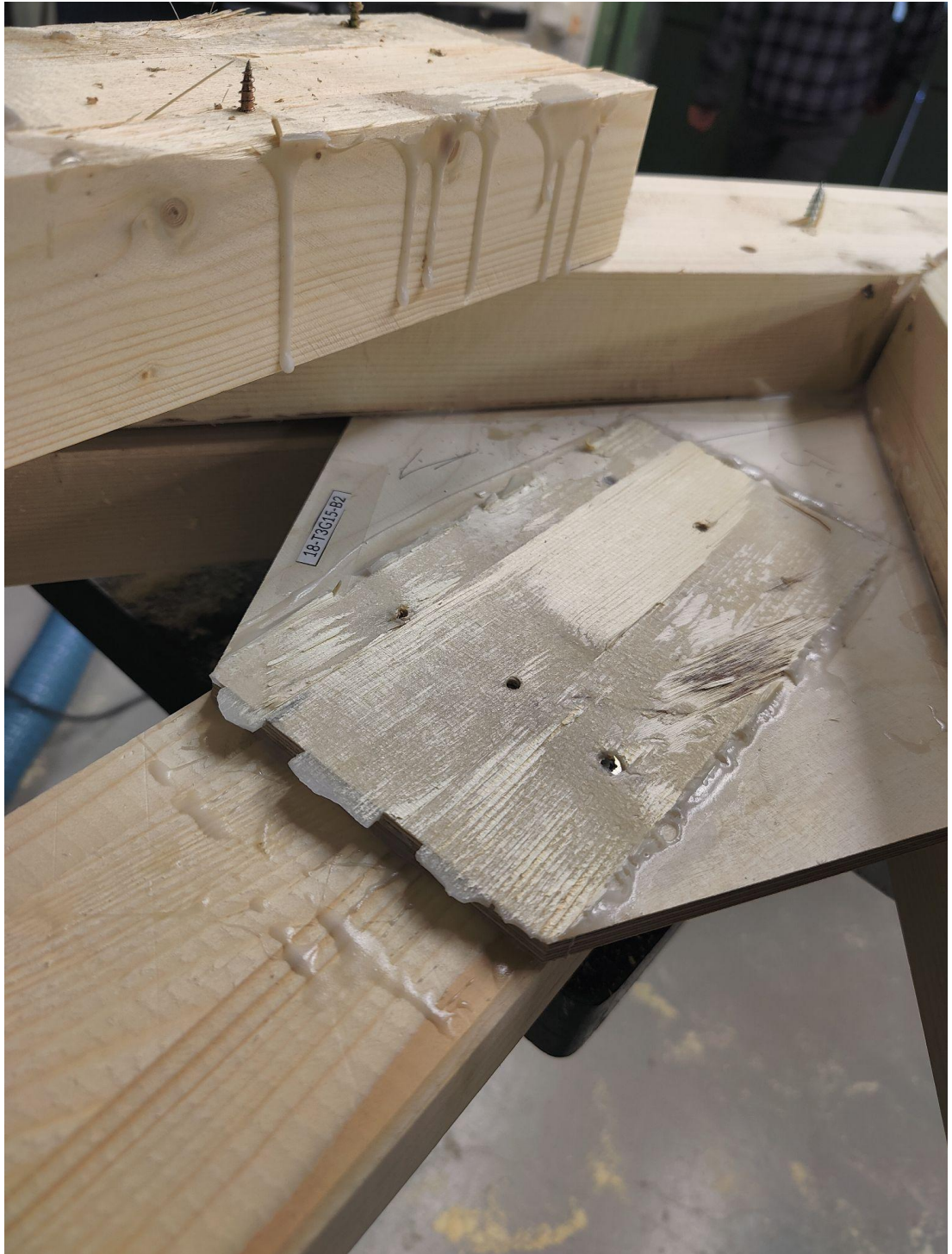
Figure A1.18.6 Glue-line failure at horizontal member
