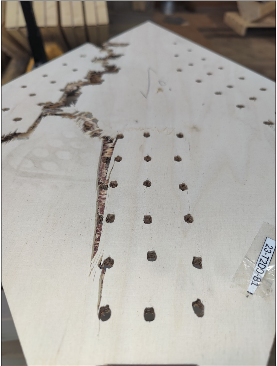
Figure A1.23.7 Failure along dowel group
