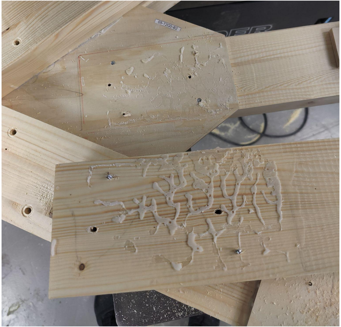
Figure A1.5.3. Especially bad glue-line
