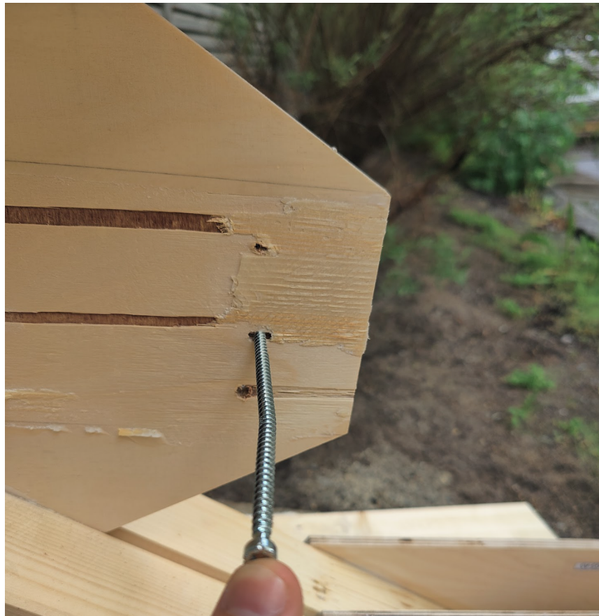
Figure A1.7.4 Deformation of nail
