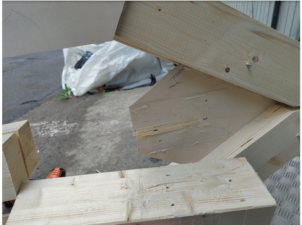
Figure A1.7.5 Glue-line failure
