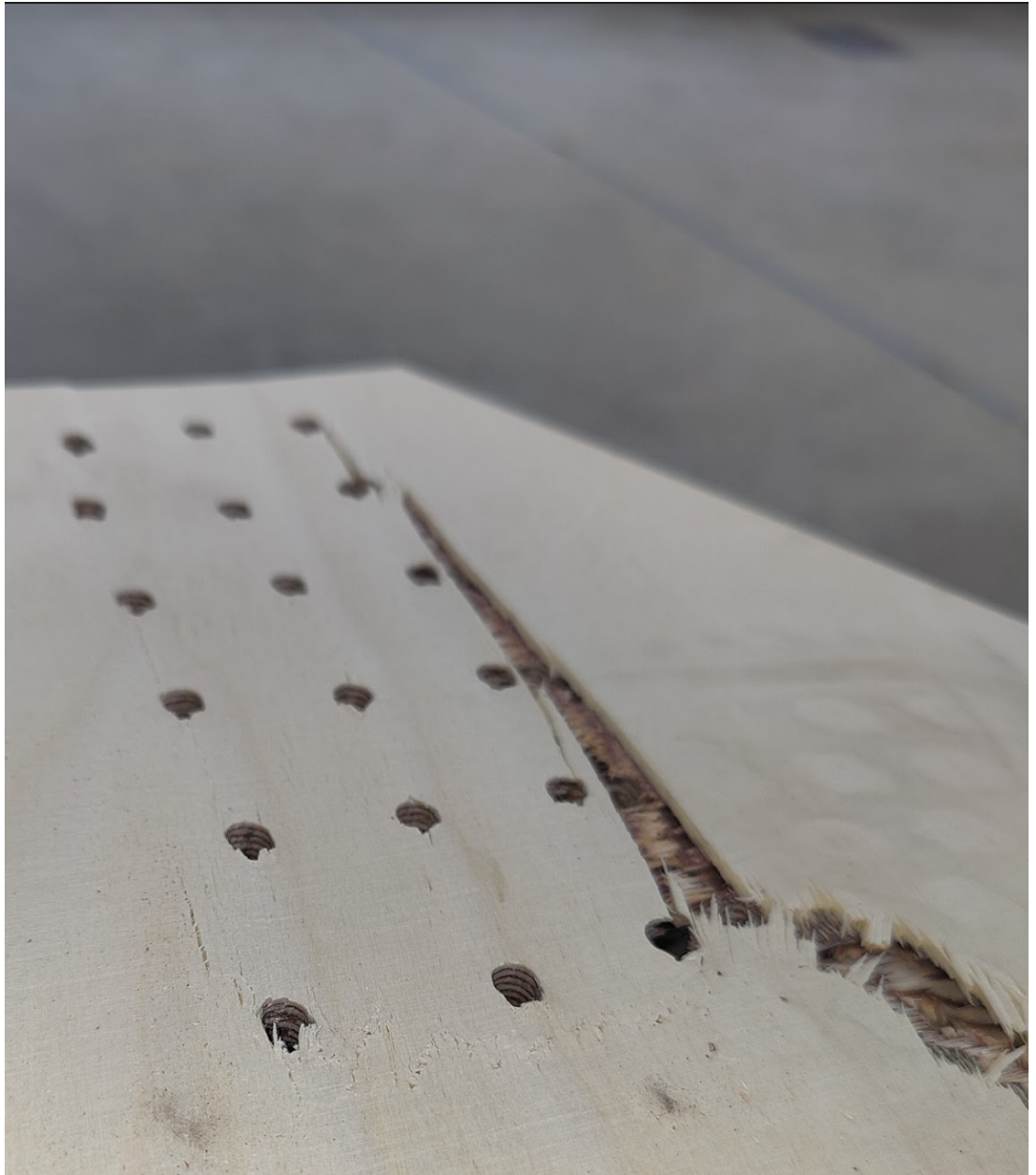
Figure A1.23.8 Compressive local buckling at dowel group
