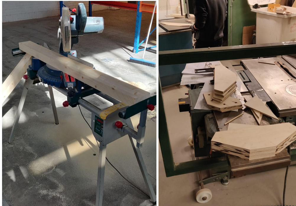
Figure 3.15. Miter saw used (to the left), and format saw used (to the right)
