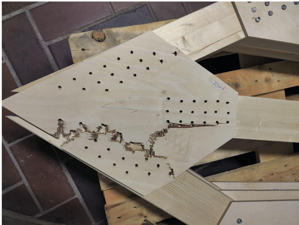
Figure A1.23.4 Plywood Failure with nails removed
