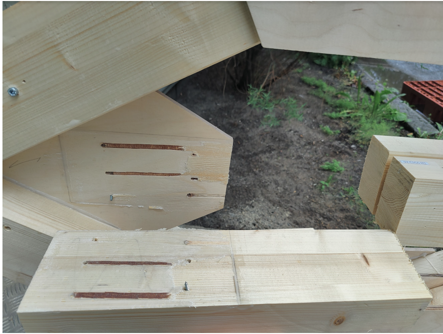
Figure A1.7.3 Glue-line failure
