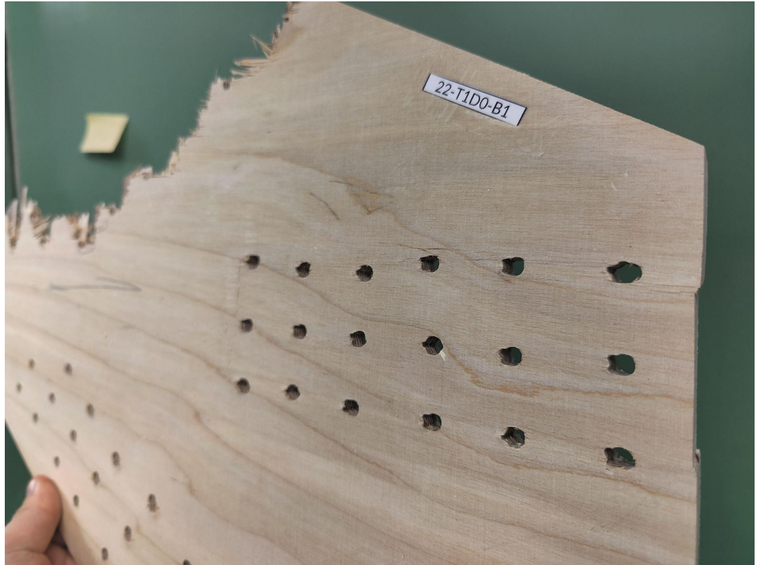
Figure A1.22.6 Plywood failure along horizontal member, compression/shear
