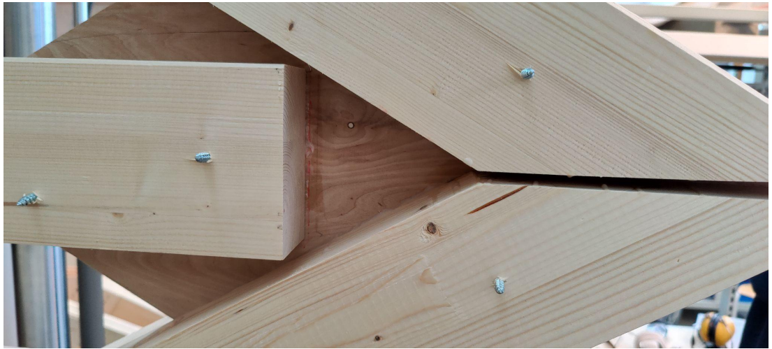
Figure A1.2.4. Location of failure 2 (glueline horizontal)
