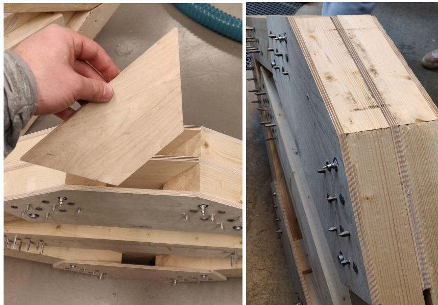
Figure 3.21. Wedges put into top and bottom of each specimen
