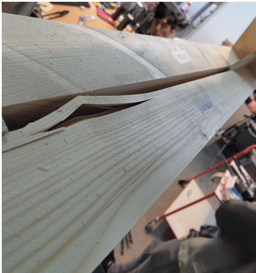
Figure A1.6.4. Timber failure in horizontal of specimen 6
