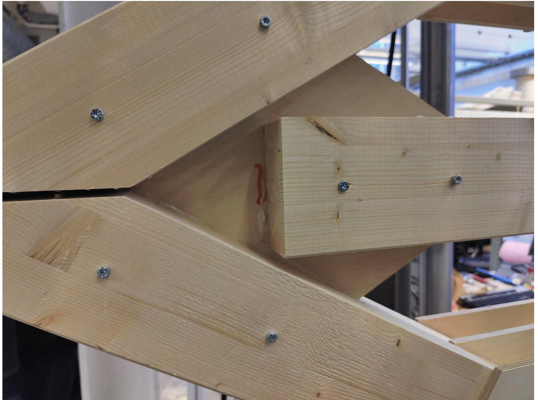
Figure A1.3.3. Location of failue 1 (glueline horizontal)
