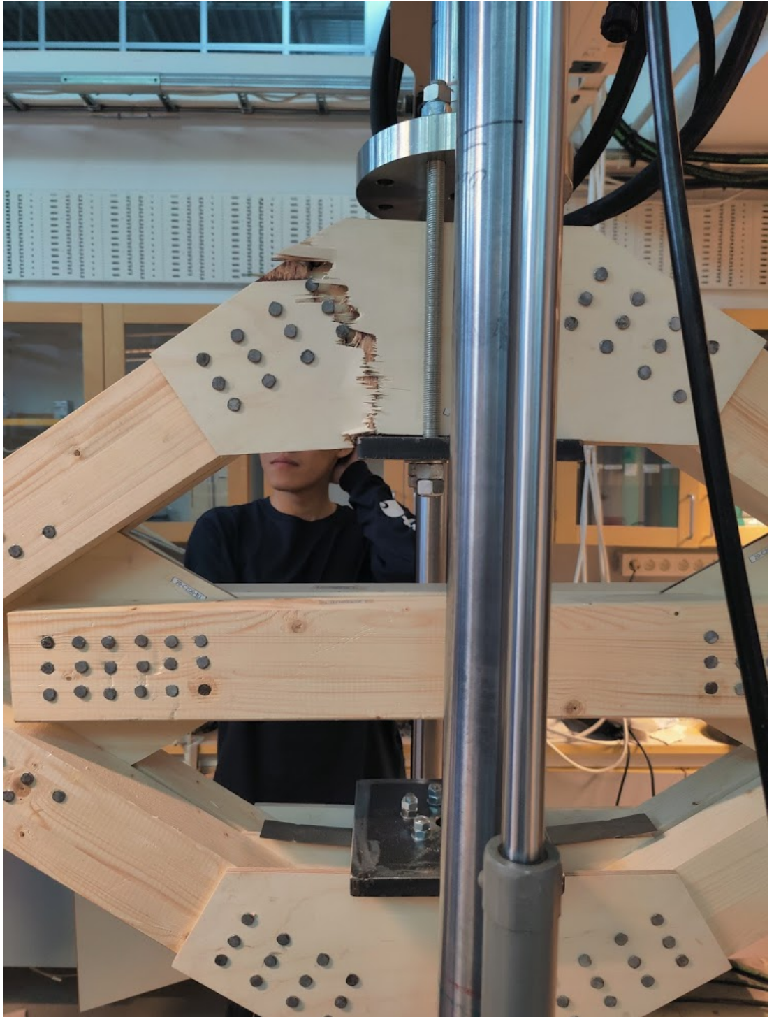
Figure A1.20.3 Plywood failure at upper gusset plates
