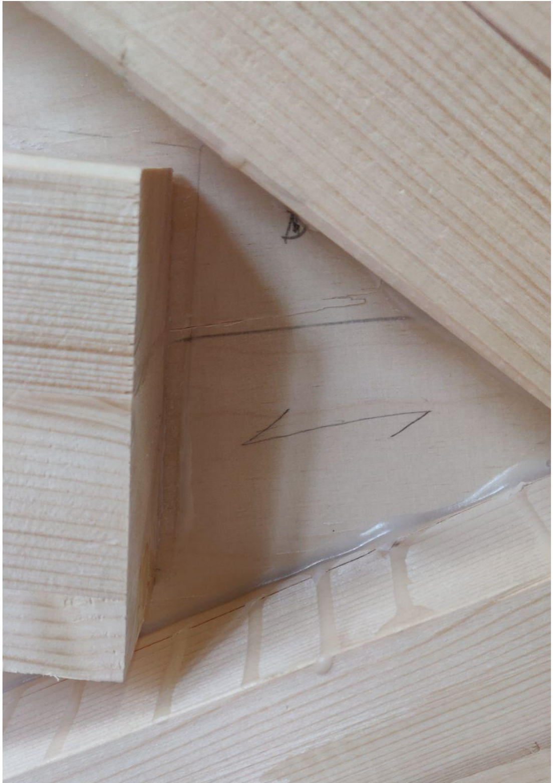
Figure A1.13.3 Glue-line failure at horizontal member, slip and small crack
