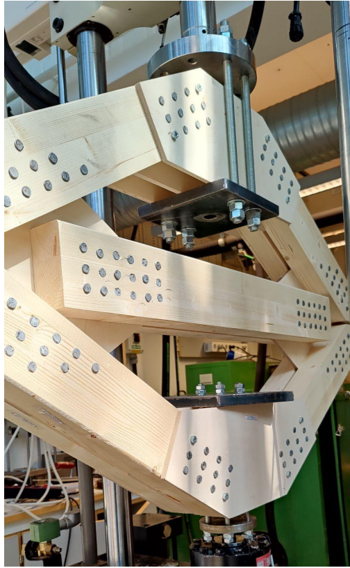
Figure 3.23. Tensile mounting supports made out of steel rods and metal plates
