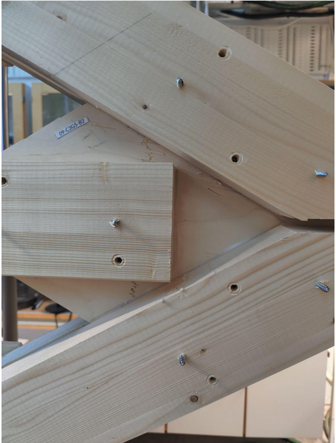
Figure A1.9.3 Tensile failure in plywood
