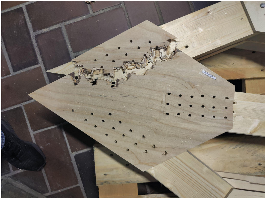
Figure A1.22.4 Plywood failure with nails removed
