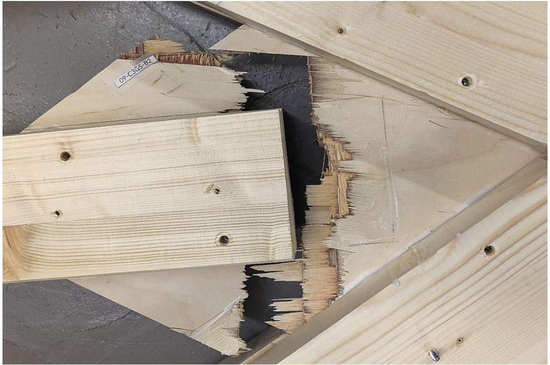
Figure A1.9.5 Plywood failure broken off after testing
