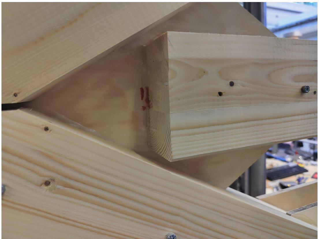
Figure A1.4.4. Glueline failure
