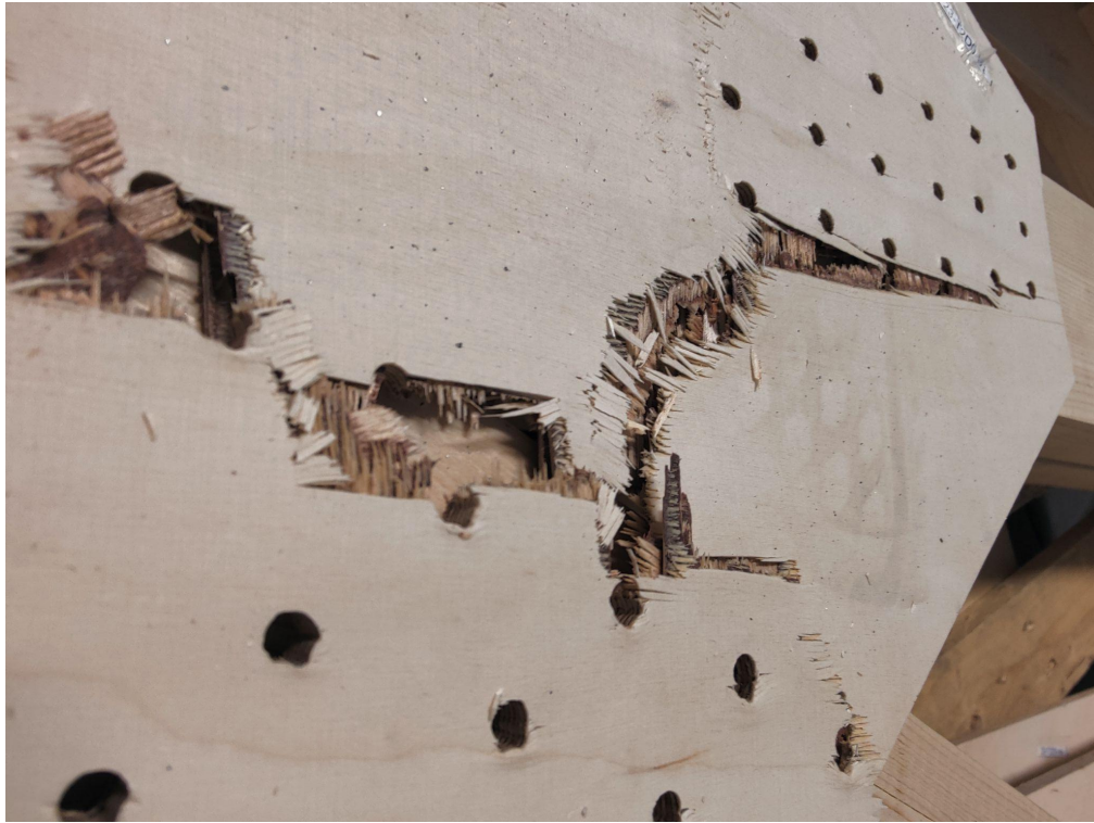
Figure A1.23.5 Plywood failure of shear crack along horizontal member
