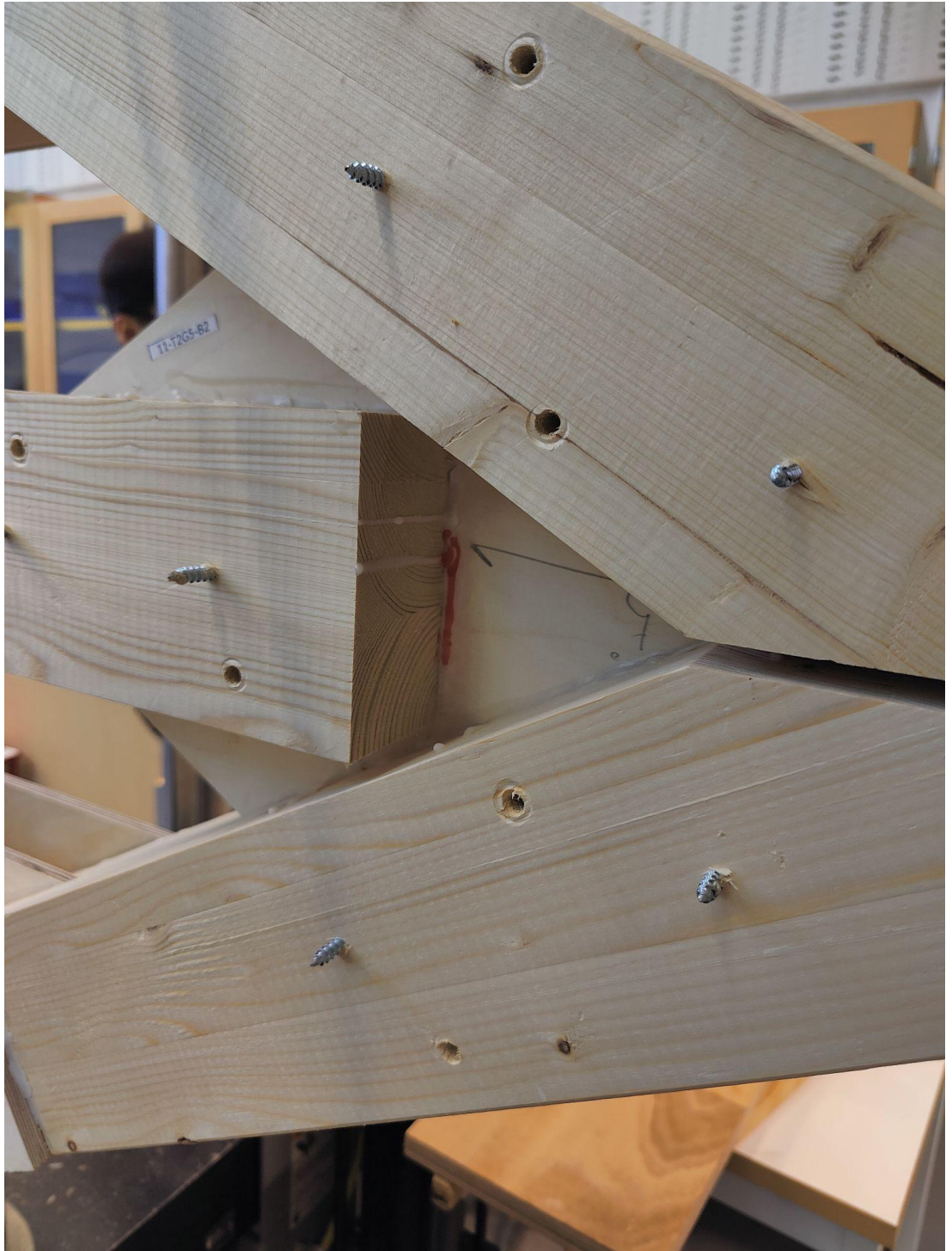
Figure A1.11.3 Glue-line failure, slip
