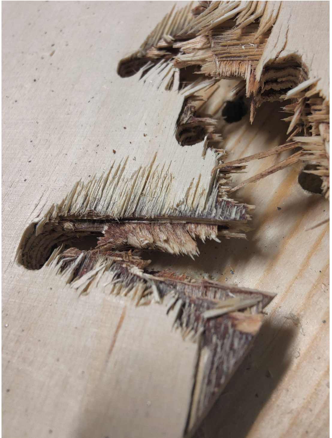
Figure A1.23.6 Failure according to Johansens' theory with nail pulled through the plywood
