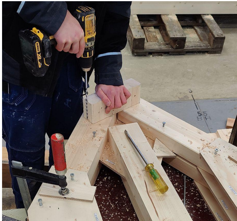
Figure 3.20. Predrilling during assembly of dowelled specimens
