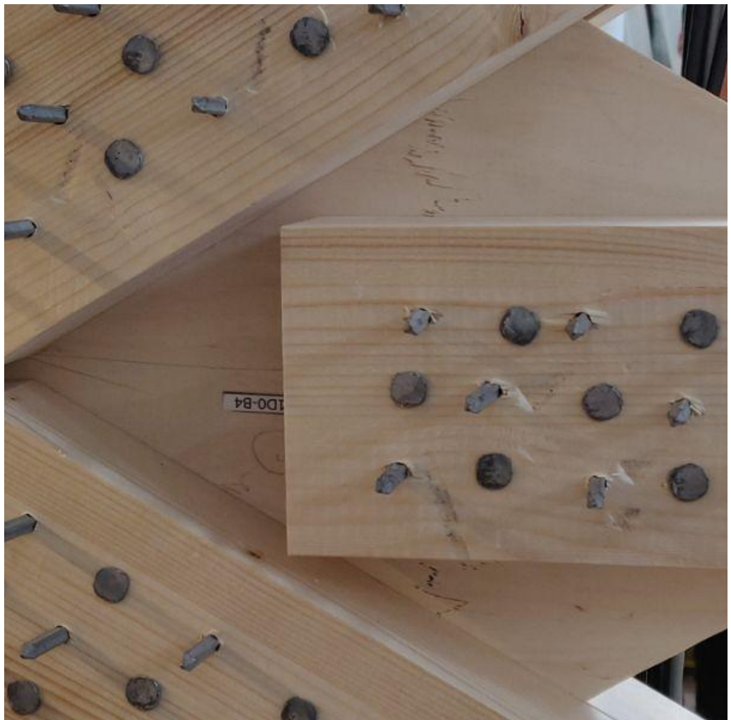
Figure A1.19.3 Plywood failure in tension around horizontal timber member
