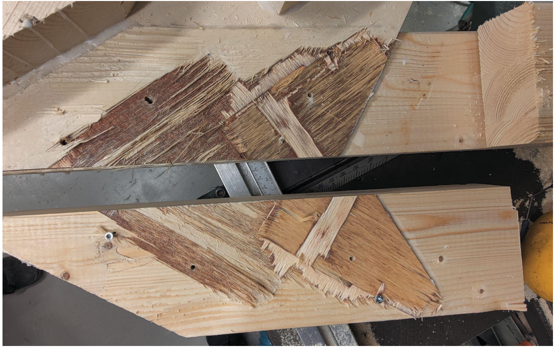
Figure A1.10.6 Glue-line failure, delamination
