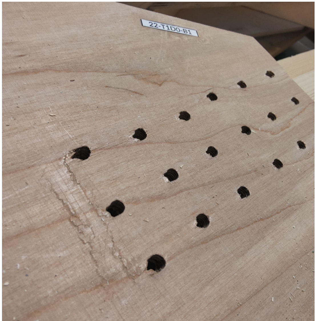
Figure A1.22.5 Plywood failure along horizontal member, local buckling
