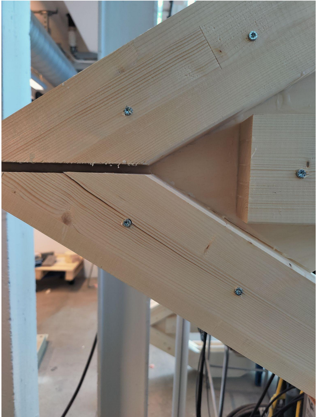
Figure A1.18.3 Shear failure in glulam
