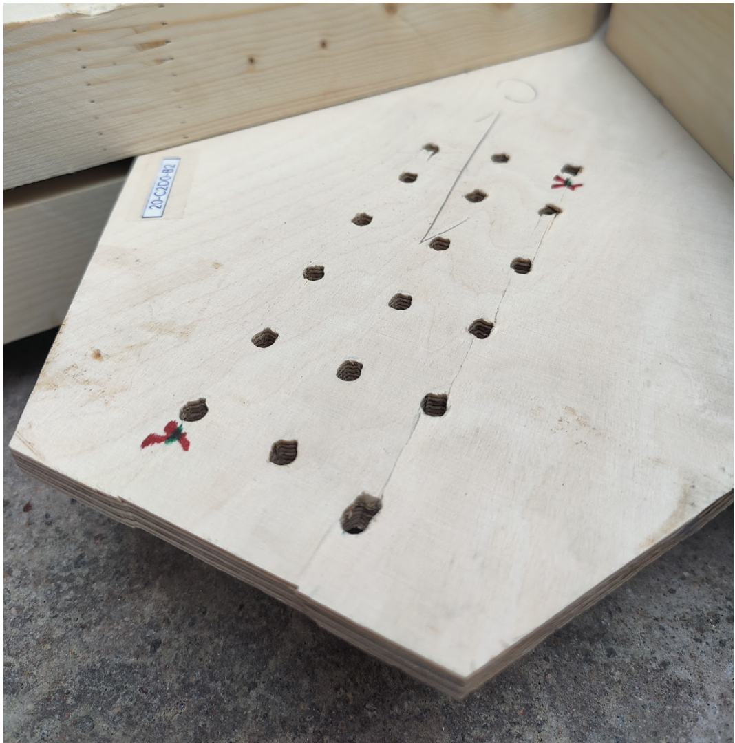
Figure A1.20.5 Failure along dowel group
