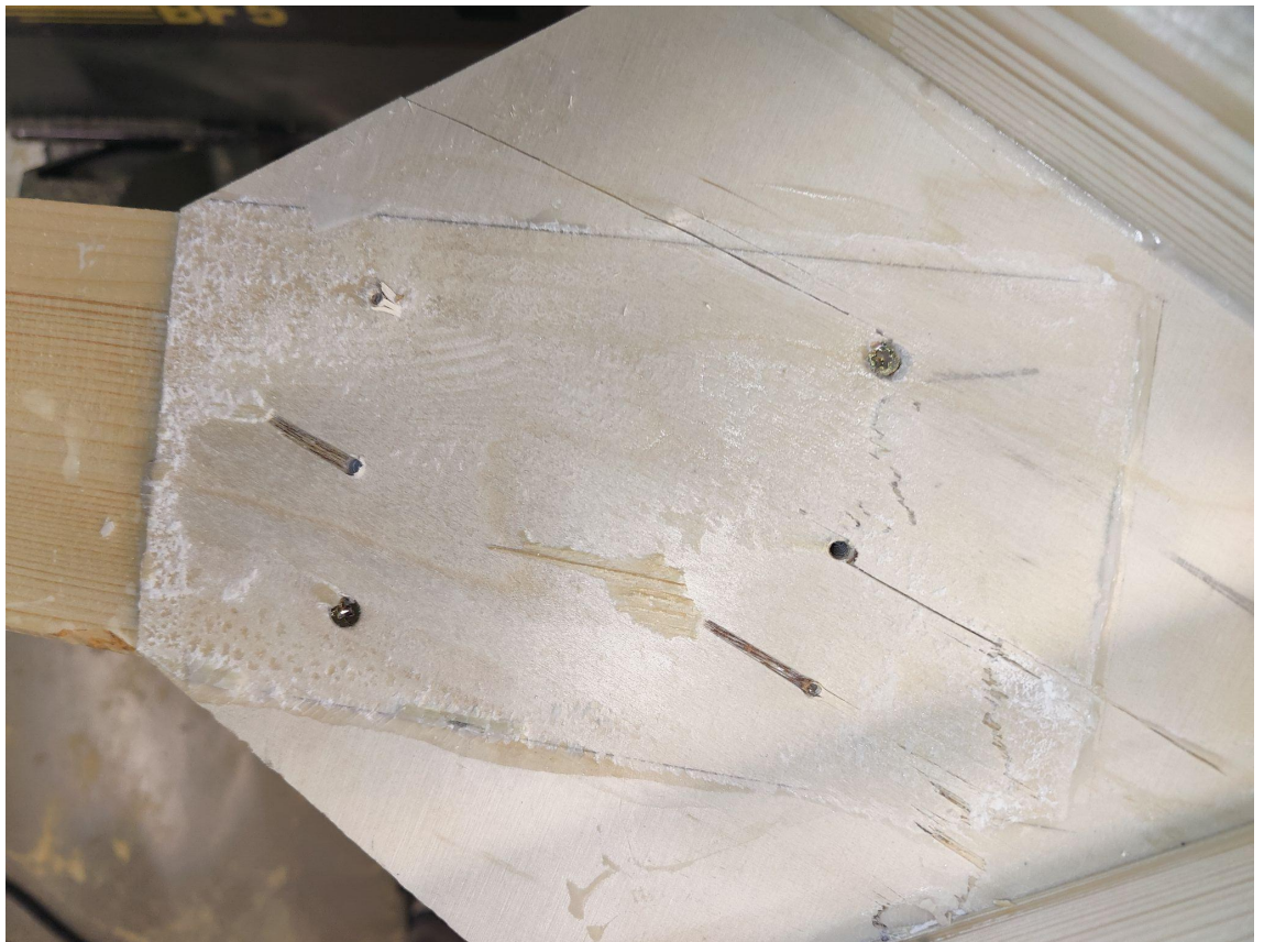
Figure A1.17.7 Glue-line failure at horizontal member
