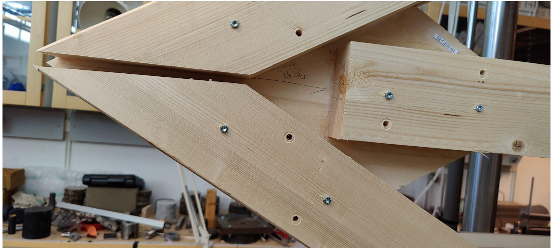
Figure A1.2.3. Location of failure 1 (glueline horizontal)
