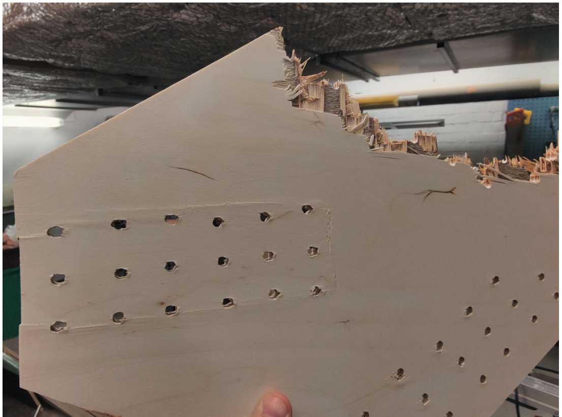
Figure A1.22.7 Diagonal plywood failure removed
