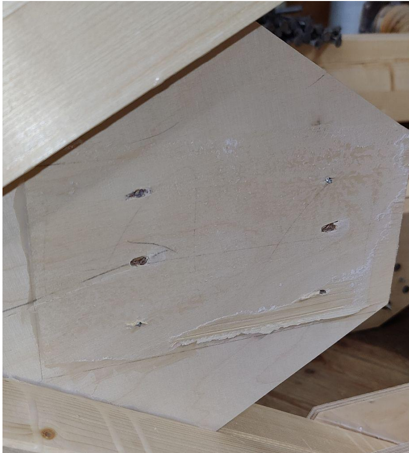
Figure A1.13.4 Glue-line failure
