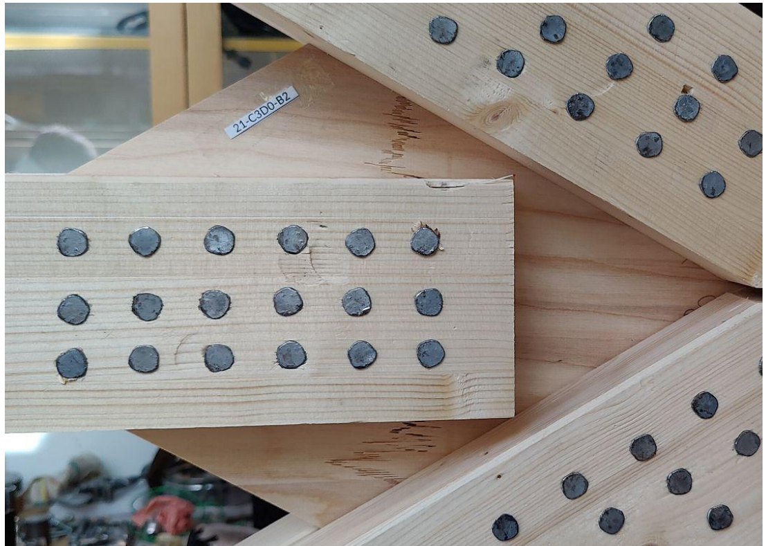
Figure A1.21.3 Plywood failure in tension at horizontal member
