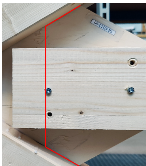
Figure 4.1. Plywood failure mode of specimen 08
