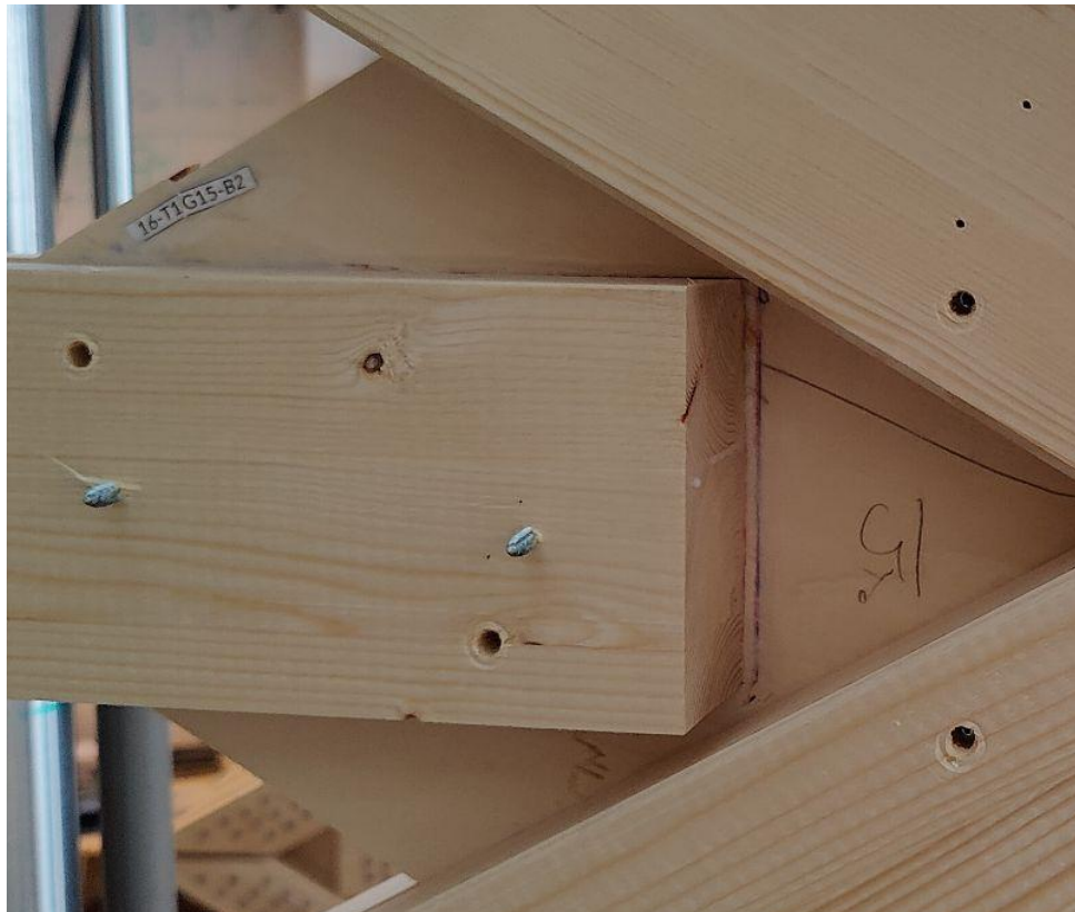
Figure A1.16.3 Tension/shear failure in plywood
