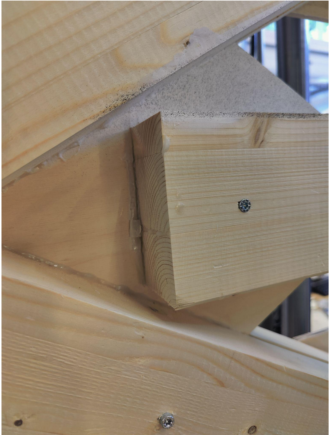
Figure A1.11.4 Glue-line failure, slip
