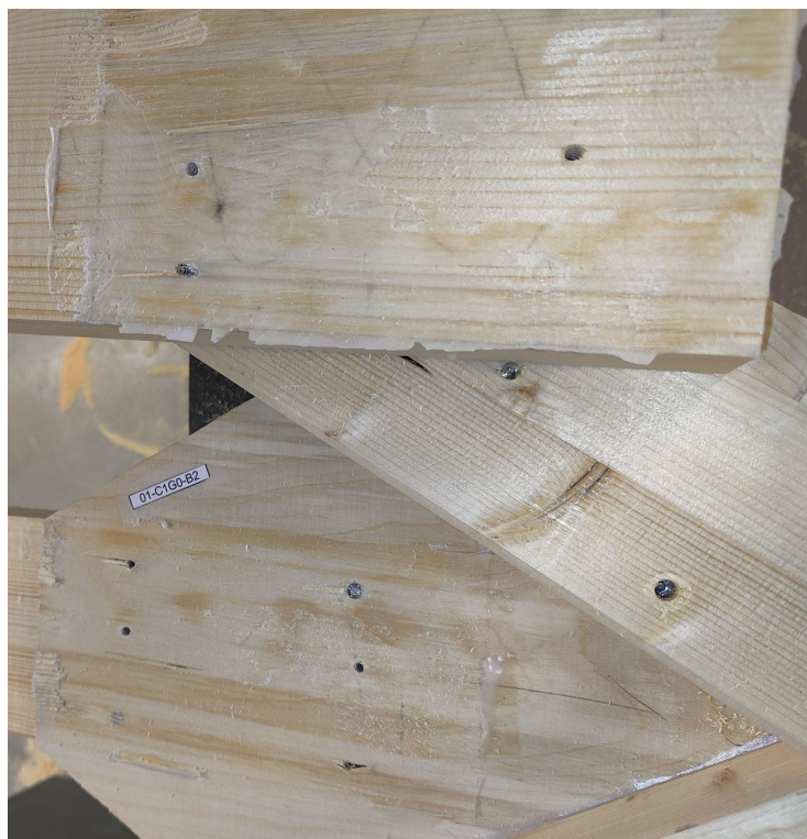
Figure A1.1.5. Glueline failure horizontal member 2
