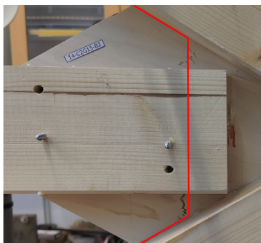
Figure 4.3. Plywood failure mode of specimen 14
