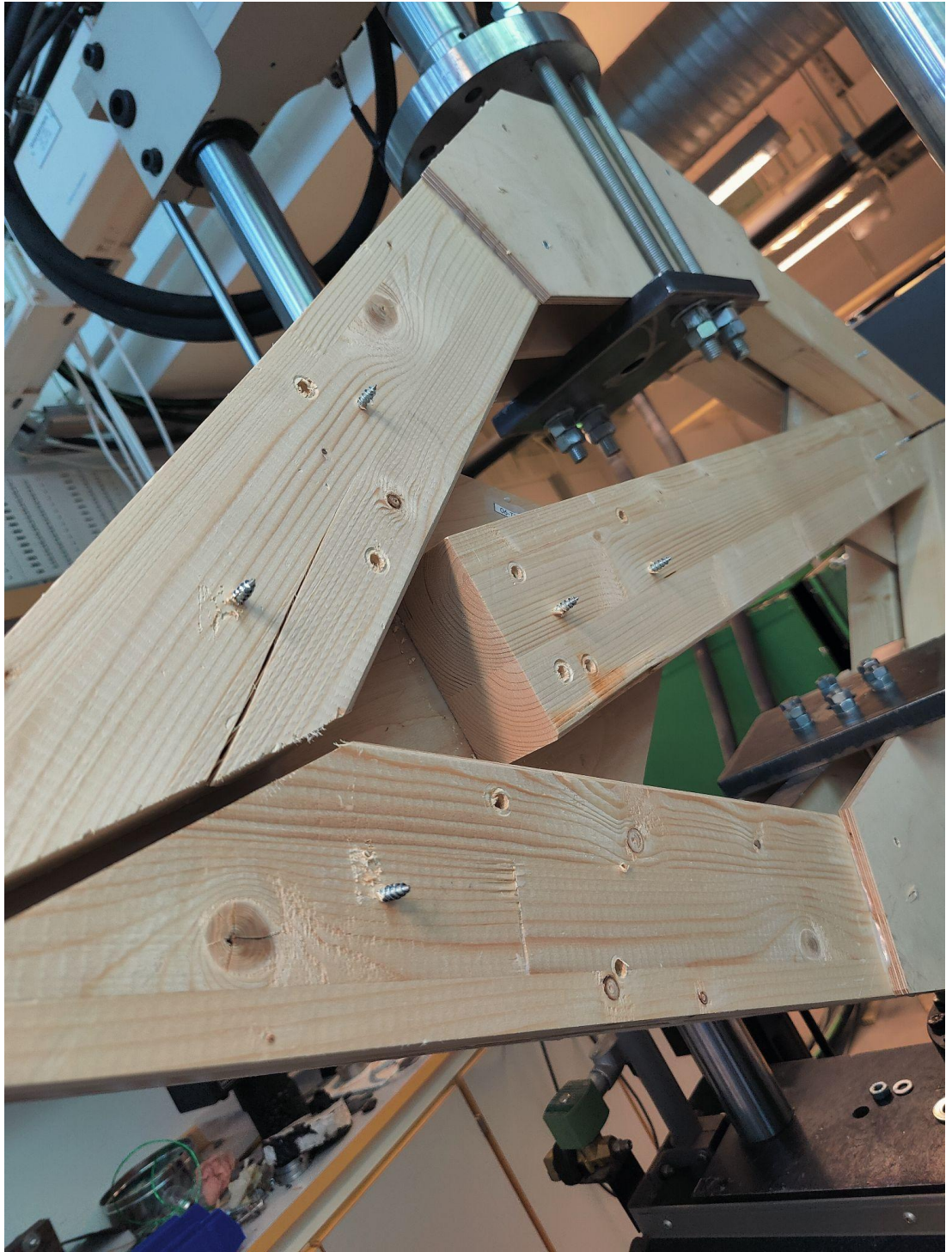
Figure A1.6.5. Timber failure in diagonal of specimen 6
