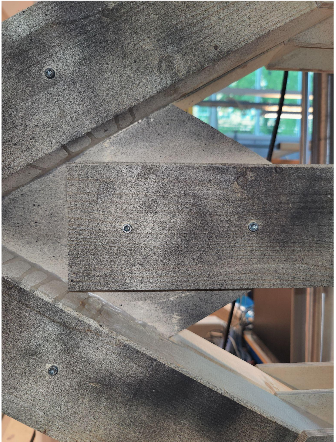
Figure A1.9.4 Plywood failure, area is painted to measure strain using camera technology
