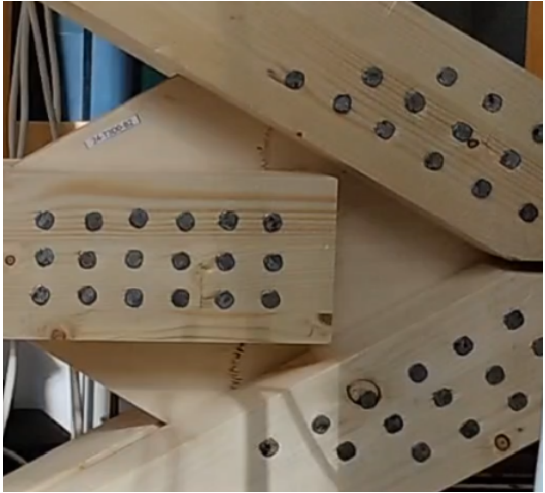
Figure A1.24.3 Plywood failure from horizontal member
