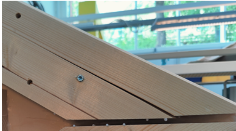
Figure A1.12.3 Shear failure in glulam
