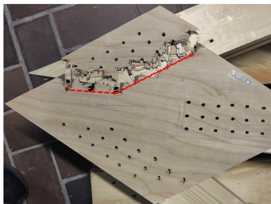
Figure 4.11. Plywood failure mode of specimen 22
