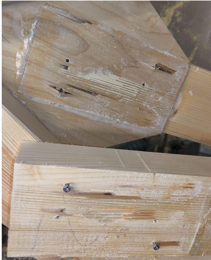
Figure A1.1.4. Glueline failure horizontal member 1
