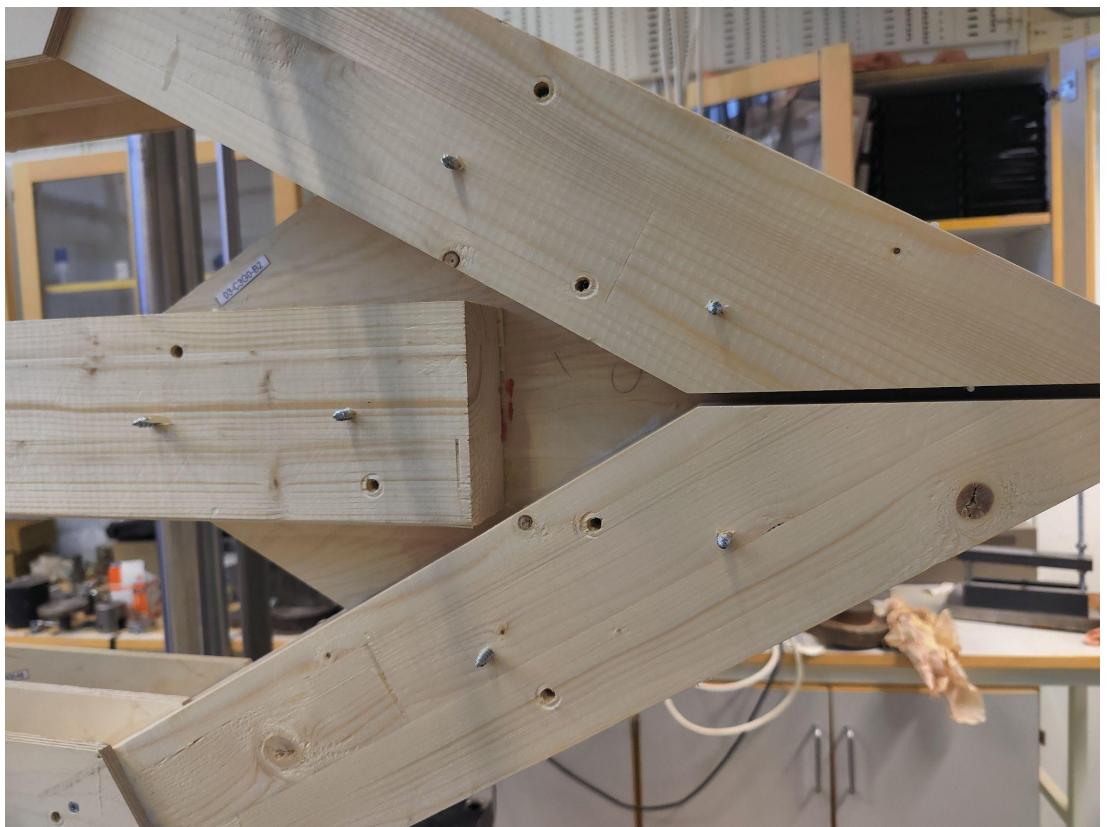
Figure A1.3.4. Location of failue 2 (glueline horizontal)
