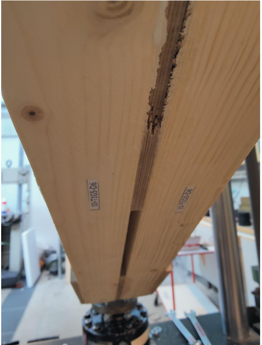
Figure A1.10.5 Failure in plywood
