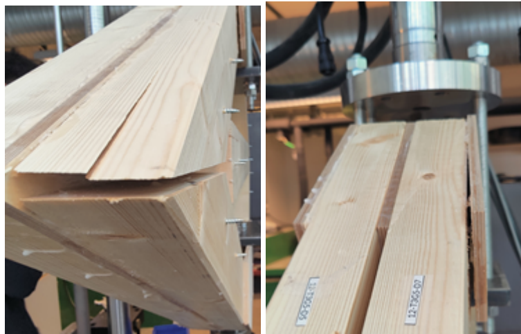
Figure A1.12.4 Shear failure in timber and glue-line failure at top gusset plate
