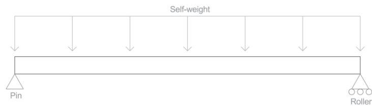
Figure 5:11 - Simply supported steel beam subjected to its self-weight
