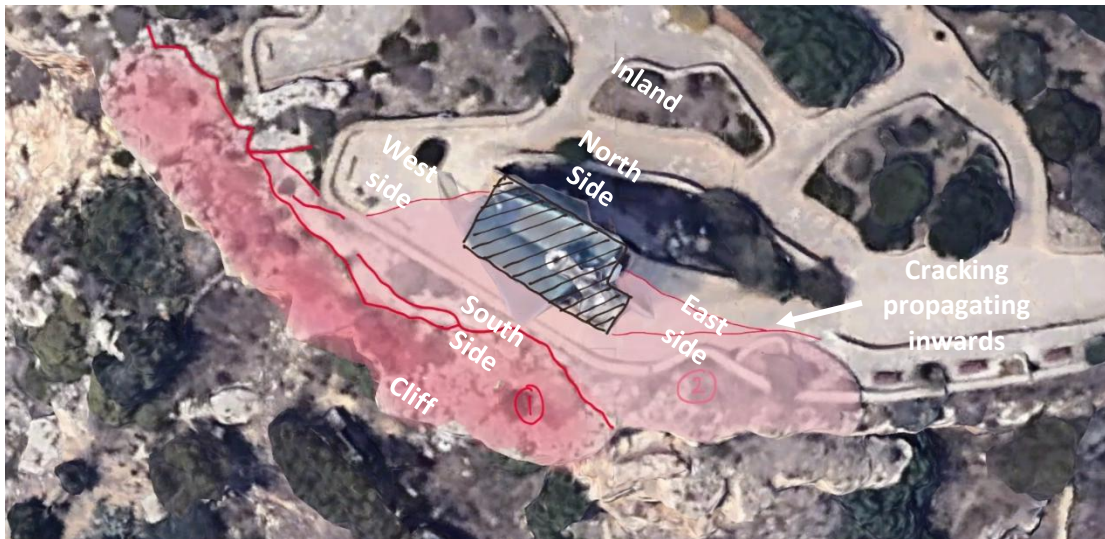
Figure 5:41 - Cracking in the ground: 1) Thick red lines indicate wide tension fissures near the cliff edge, 2) Thin light red lines represent narrower cracks beneath the structure
