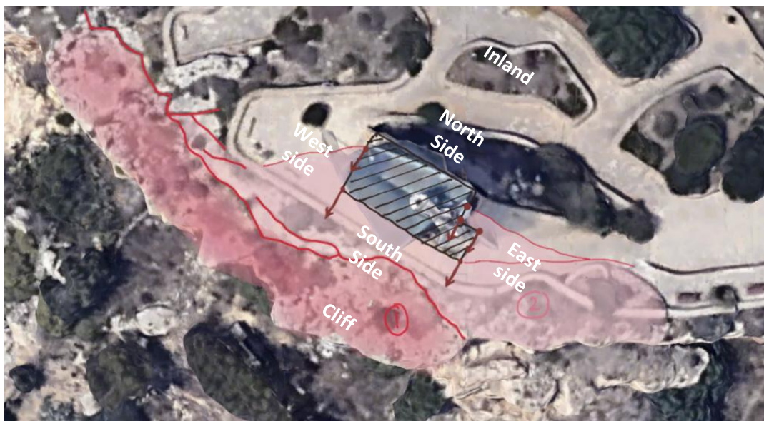
Figure 5:44 - Ground crack mapping and locations within the structure where nodal deformations are applied
