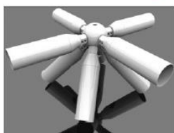
Grid Shell Node Types Spherical Node S
