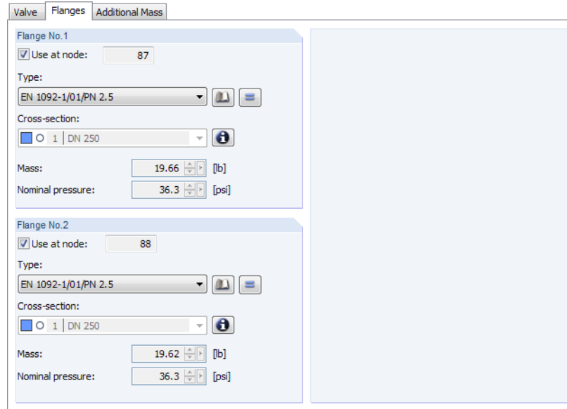
Figure 2.19: Dialog box New Valve , tab Flanges
