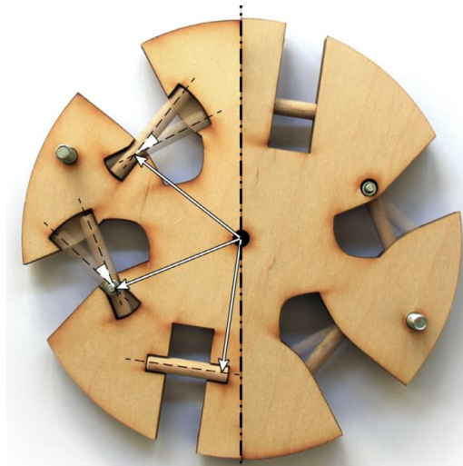
Figure 28. Experimental multi-member hub joint developed for the deployable triangulated scissor grid system [4].
