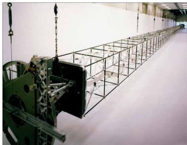
Figure 10. SRTM (Shuttle Radar Topography Mission) mast fully deployed (JPL) [9].
