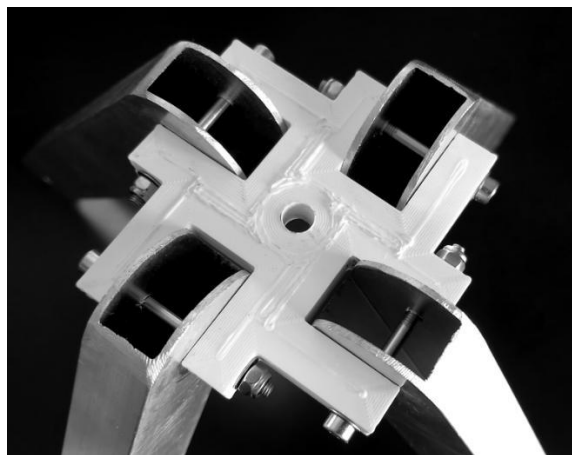
Figure 14. Example of a hub type joint [13].
