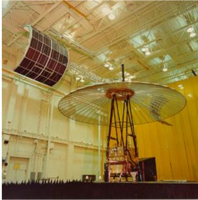
Figure 9. ATS-6 during radio-frequency tests (NASA) [8].
