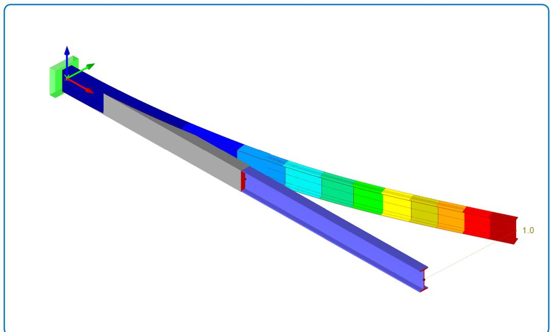
**Figure 2:** Results in RFEM 5 / RSTAB 8 – First eigenvector, load factor  $f = 0.708$ .
