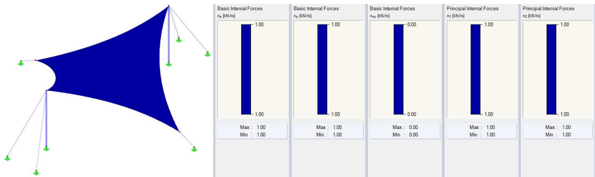
Fig. 7 – Basic internal forces n_x, n_y, n_{xy} and the principal internal forces n_1, n_2
