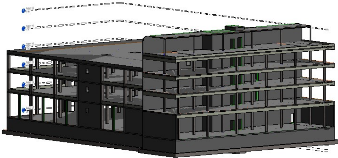
Pic.1. Model of the designed building made in program Revit
