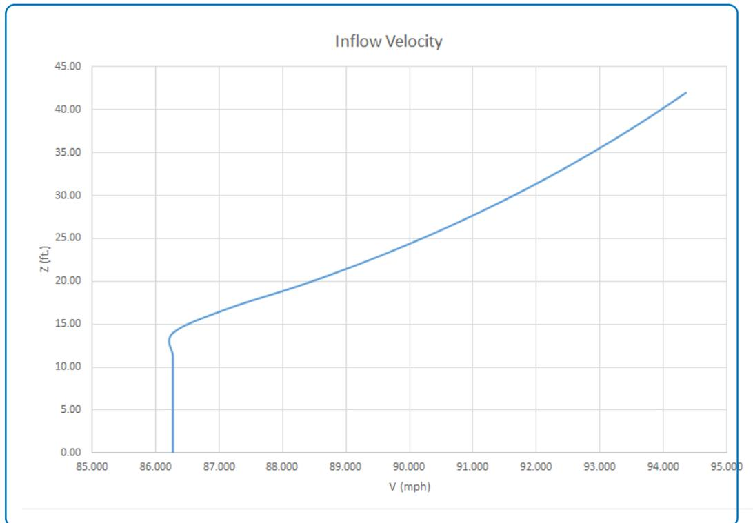
**Figure 2:** Inflow velocity according to ASCE/SEI 7-16 (exposure category D, basic wind speed 100 mph)
