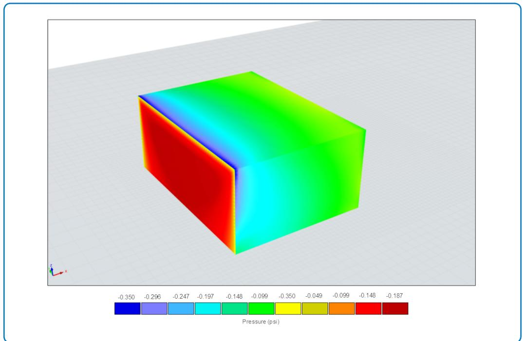
**Figure 4:** RWIND Simulation – Surface pressure
