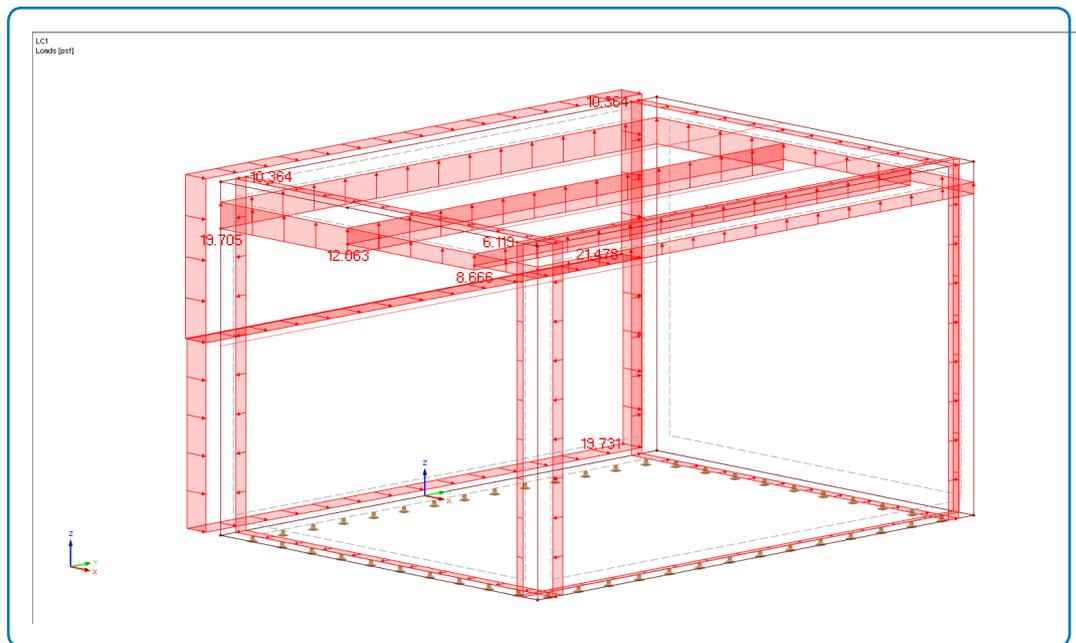
**Figure 3:** RWIND Wind Load Generator – LC1 Surface pressure
