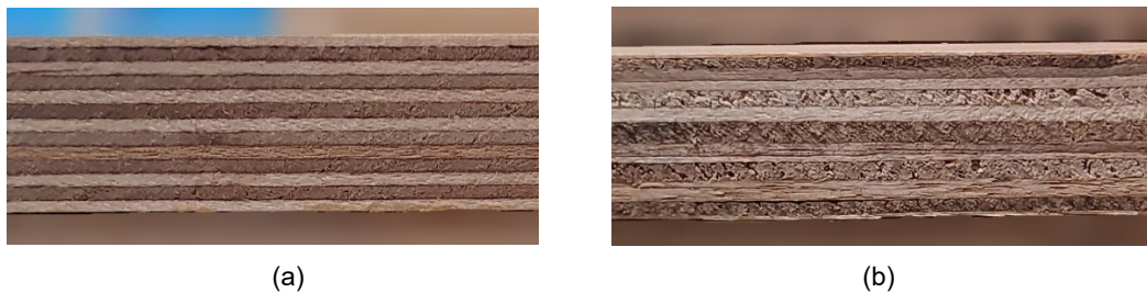
Figure 3-2: Plywood: (a) high-quality (grade B) and (b) low-quality (grade C)
