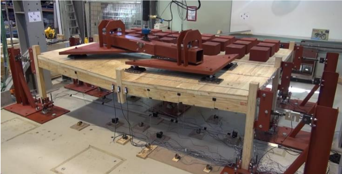
Figure 2-7: Test setups: 3D post-and-beam frame (Lyu et al., 2018) (Reprinted with permission)
