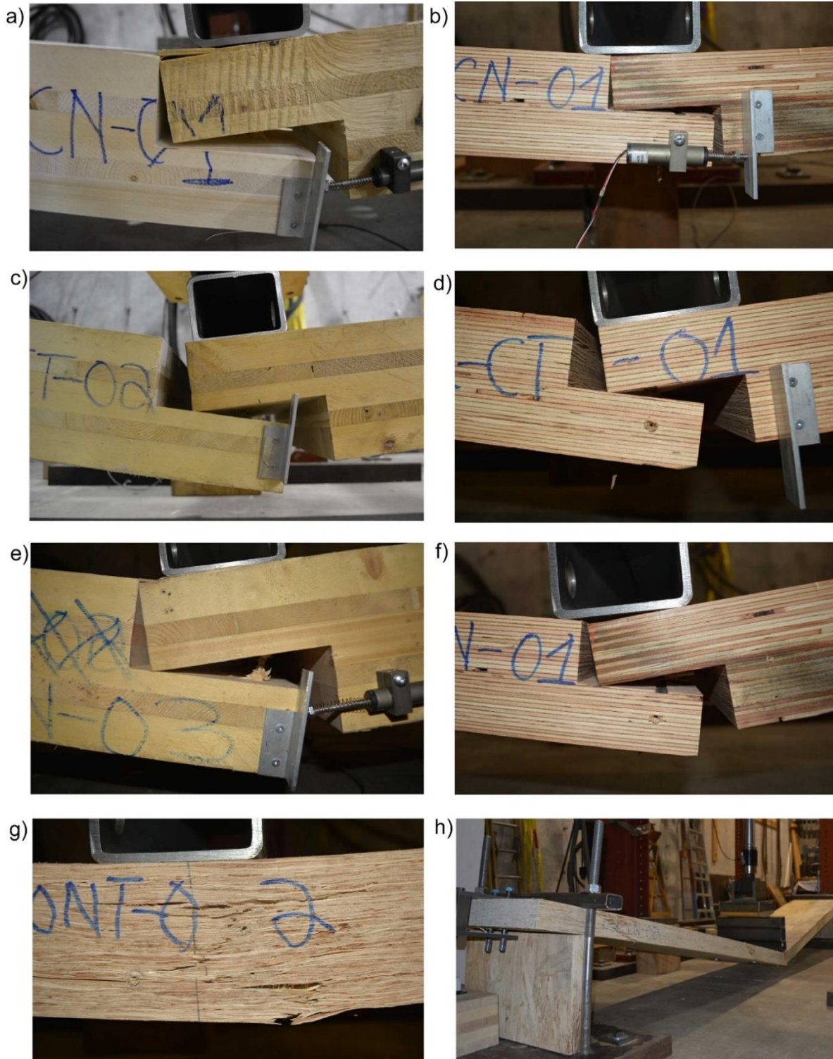
Figure 8-9: Failure modes at mid-span: (a) at \Delta = 70\text{mm} for CI CLT assembly; (b) at \Delta=45\text{mm} for CI LVL assembly; (c) at \Delta=150\text{mm} for CI-Trad CLT assembly; (d) at \Delta=150\text{mm} for CI-Trad LVL assembly; (e) at \Delta=250\text{mm} for CI-Novel CLT assembly; and (f) at \Delta=250\text{mm} for CI-Novel LSL assembly
