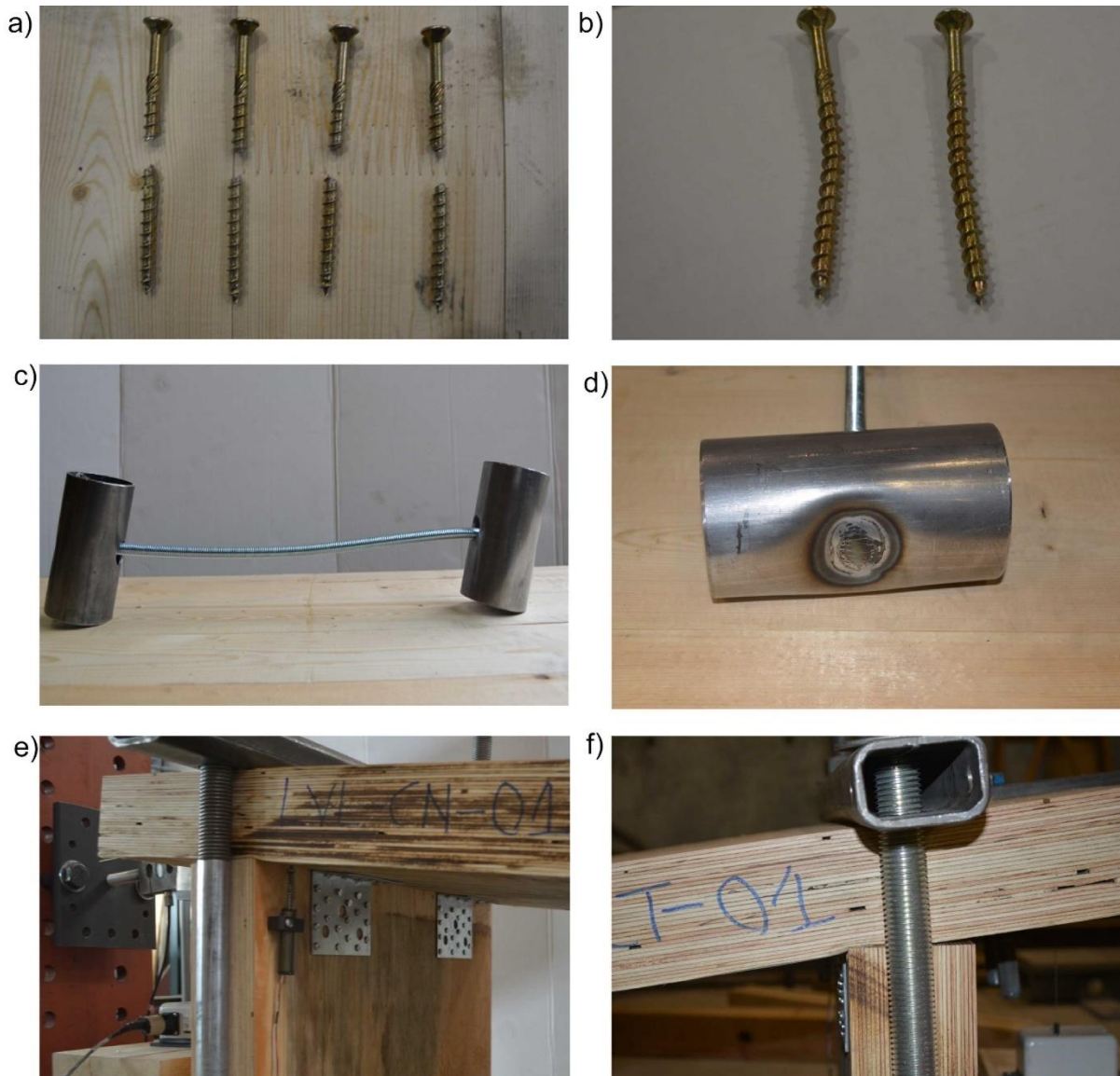
Figure 8-10: Failure modes: (a) Shear failure of STRs for C1-Trad; (b) Excessive deformation of STRs for C1-Novel; (c) Deformation of steel tube and rods; (d) Inelastic buckling of steel tube; (e) Deformation of angle brackets; and (f) Compression perpendicular to the grain of mass-timber floor
